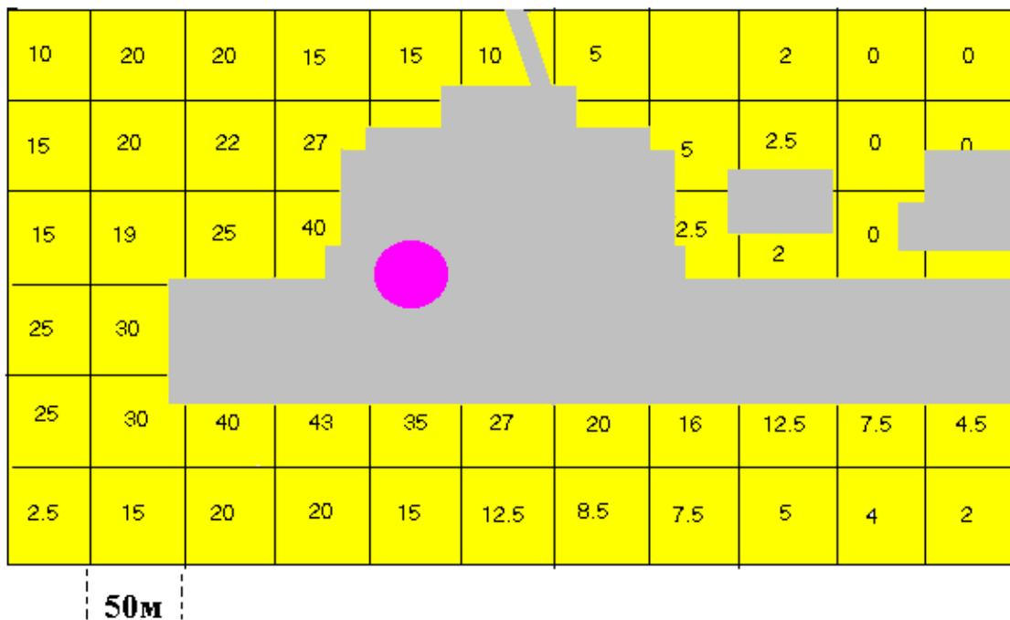
FIG. 5. Distribution of spent fuel fallout at the Shelter site (in kg per 50 x 50 m<sup>2</sup>).
