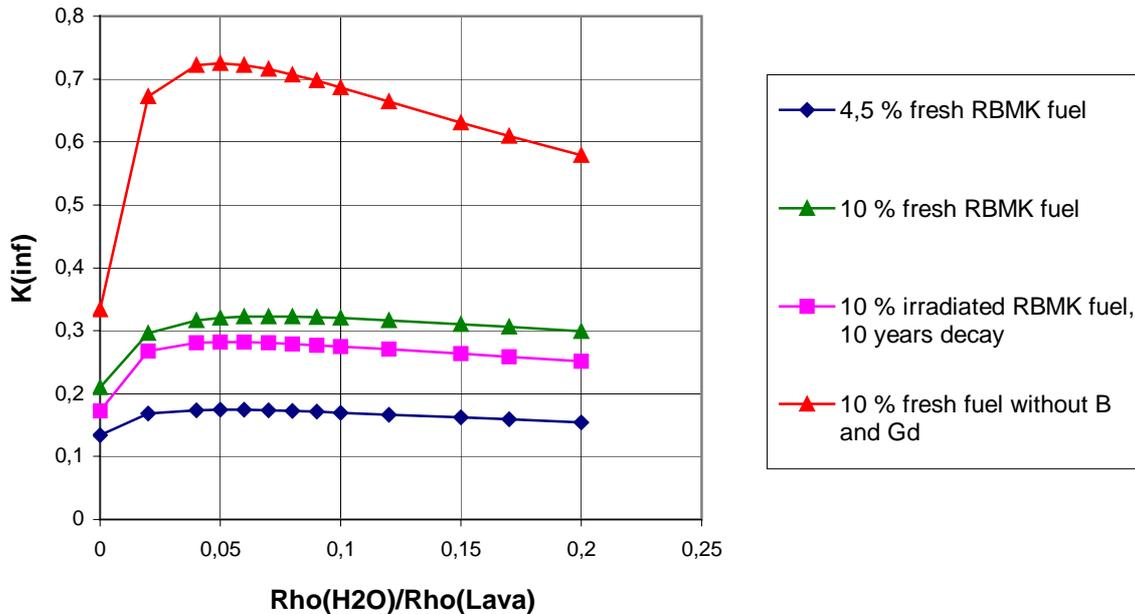
FIG. 2. Neutron multiplication factor  $k_{inf}$  for fuel lava in room 304/3 versus water contents.
