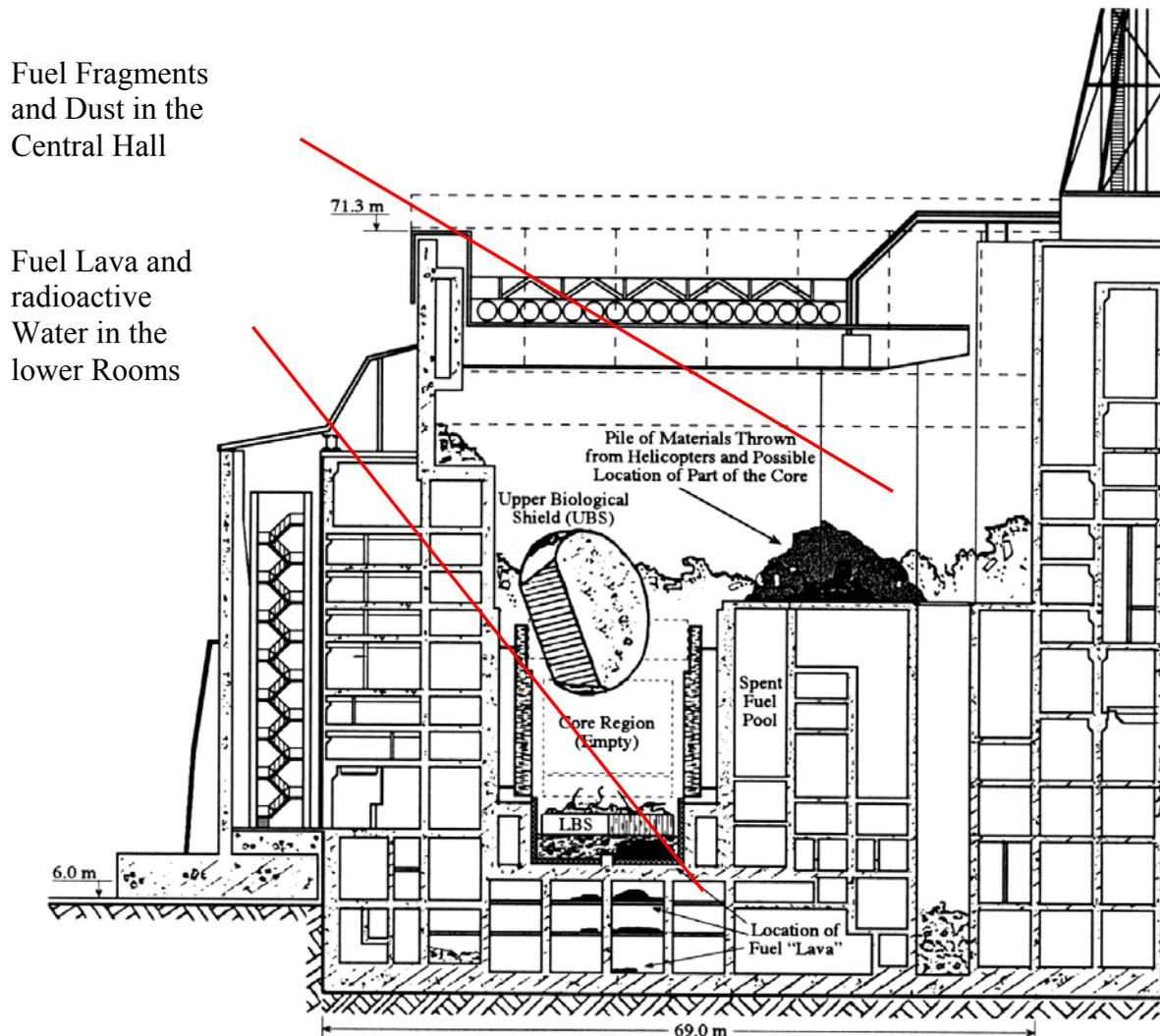
FIG. 1. Scheme of the cross section West-East of the Chernobyl object Shelter.
