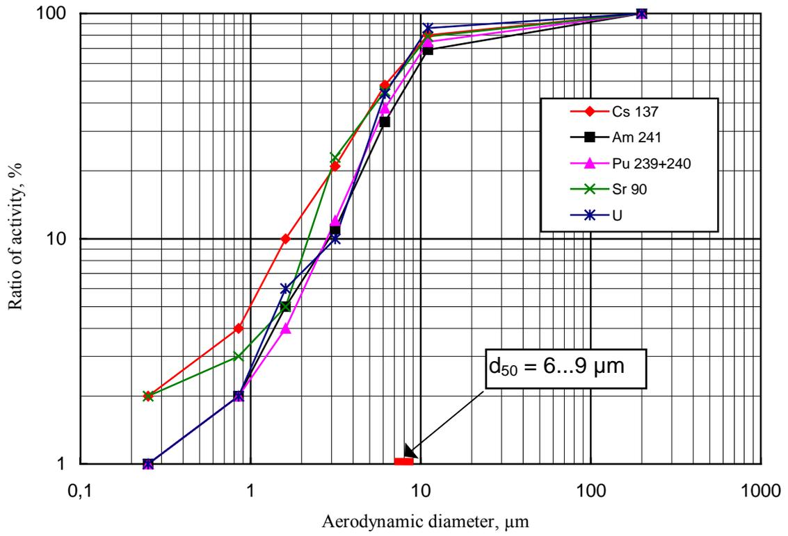
FIG. 3. Cumulative activity distribution depending on the AED of the fuel dust particles.
