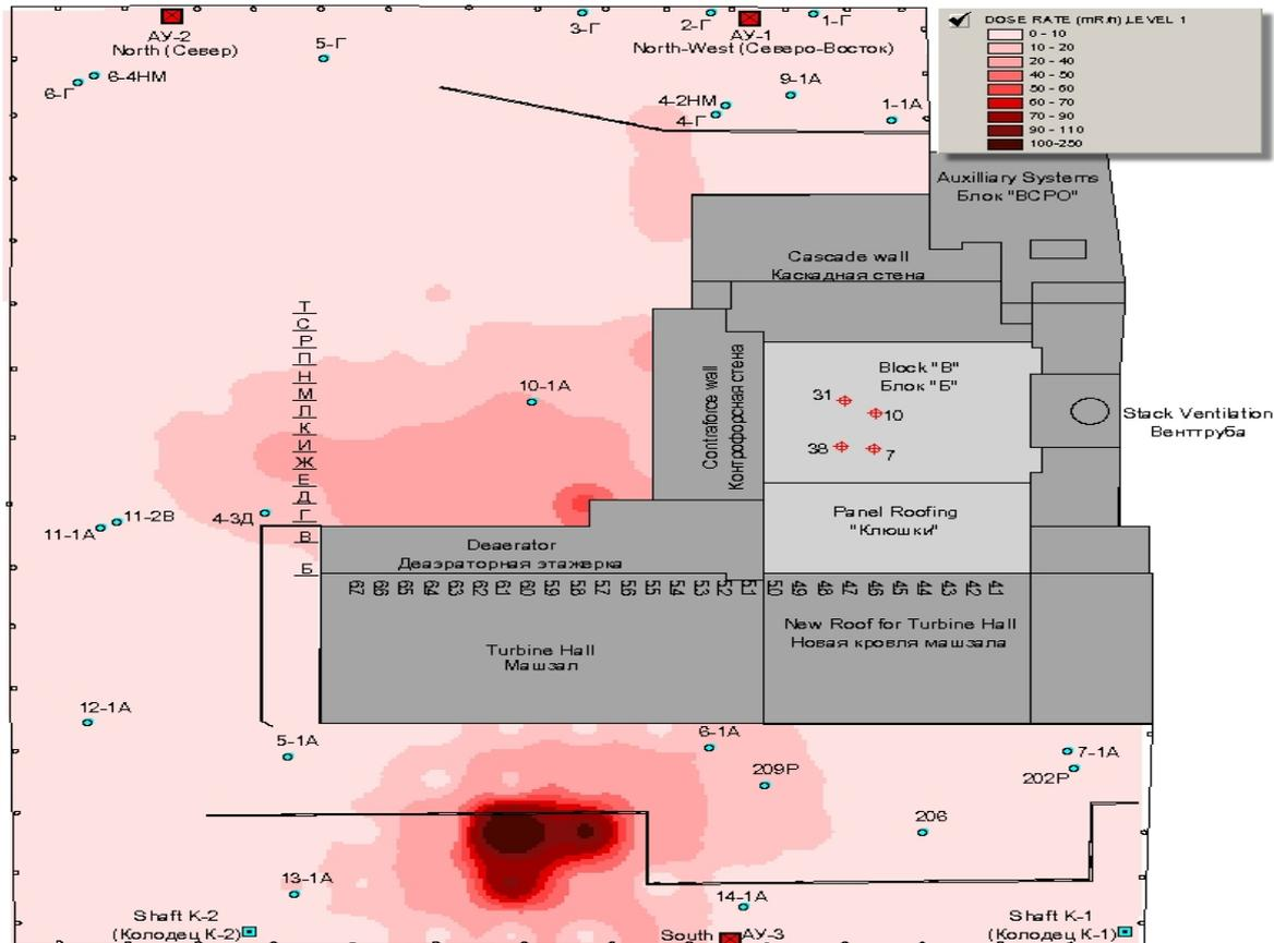
FIG. 6. Dose rate 1 m above ground at the Chernobyl object Shelter site in 2002, aspiration units AU-1 to AU-3 for aerosol sampling (red), bore holes for ground water inspection (blue).
